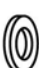
12 RONDELLA Ø8x14mm WASHER Ø8x14mm RONDELLE Ø8x14mm SCHEIBE Ø8x14mm ARANDELA Ø8x14mm Q.TY n.4
